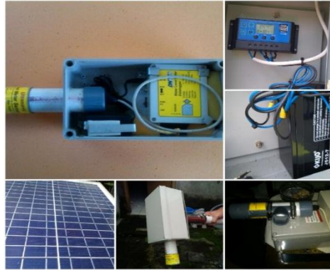
Gambar 1 Instrumen tinggi muka tipe ultrasonic portable water level recorder .
